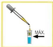
1 – Heat the oil around 120°C (high enough to melt the product inside the tube). Fill the tube 'till the lower label limit, using the filler (supplied with the kit).
