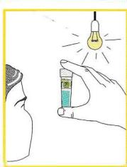
3 – Wait 2 minutes and hold the tube on the counter-light. Compare with the chromatic scale on the label.
